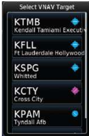
Figure 15-9 Select VNAV Target Waypoint List
