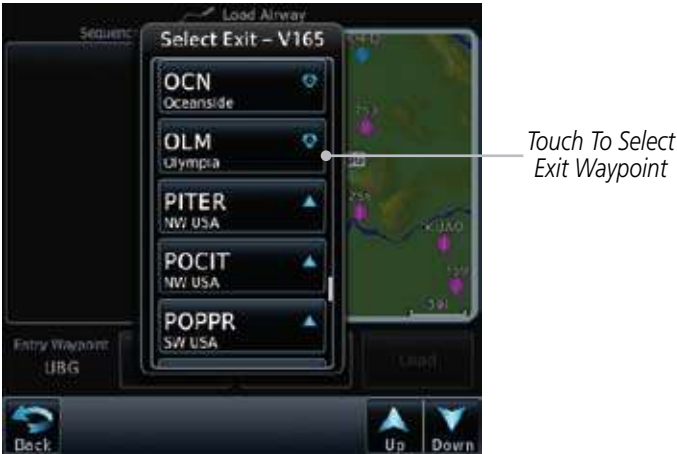
Figure 4-19 Select an Exit Waypoint for the Airway
