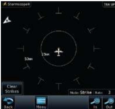
Figure 12-42 StormScope 360° and Arc Display Views
