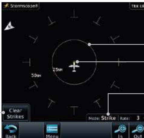
Figure 12-40 StormScope Display (360° Display View Shown)
