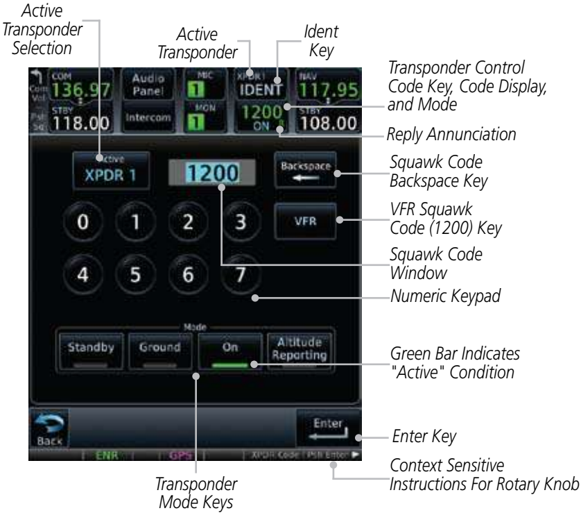
Figure 2-1 XPDR Control Display
