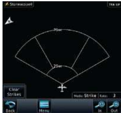
Figure 12-42 StormScope 360° and Arc Display Views
