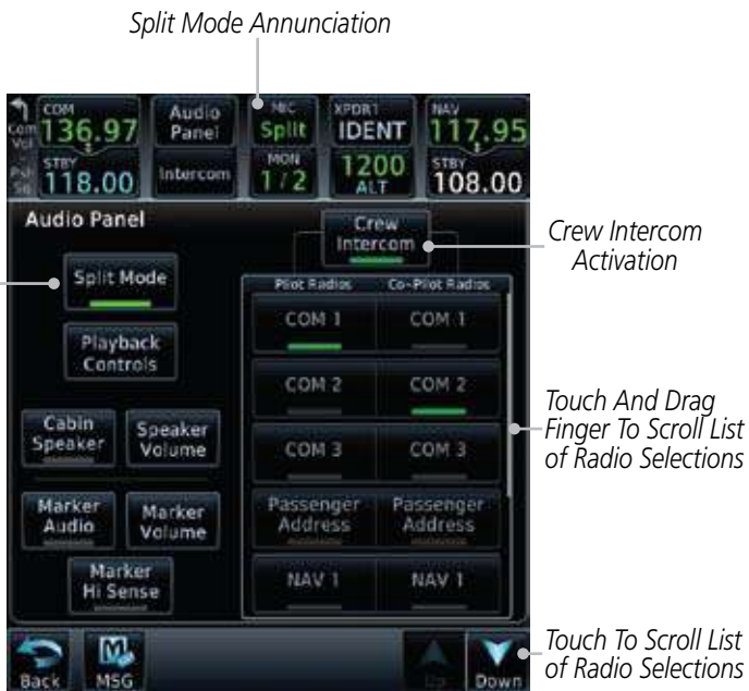
Figure 2-15 Audio Panel Split Mode Controls
